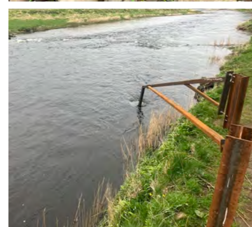
Below Left: The new ARIS SONAR deployment structure. The height of the ARIS can be adjusted from the river bank and is designed to swing into the bank if struck by very large debris during a flood.
