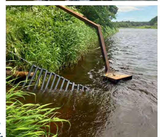
Below Left: The new ARIS SONAR deployment structure. The height of the ARIS can be adjusted from the river bank and is designed to swing into the bank if struck by very large debris during a flood.
