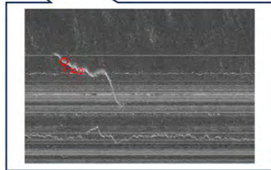
A snap shot of the Aris Fish software interface used for processing the SONAR footage. Highlighted in the callout box is the typical echogram signature of a 74cm salmon and below it a small stationary trout.
