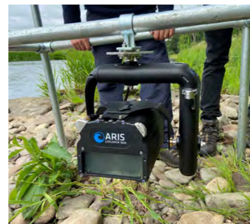
Left: The ARIS 1800 suspended from the temporary scaffolding frame with the AR2 rotator arm that allows remote adjustment of camera both vertically and horizontally.
